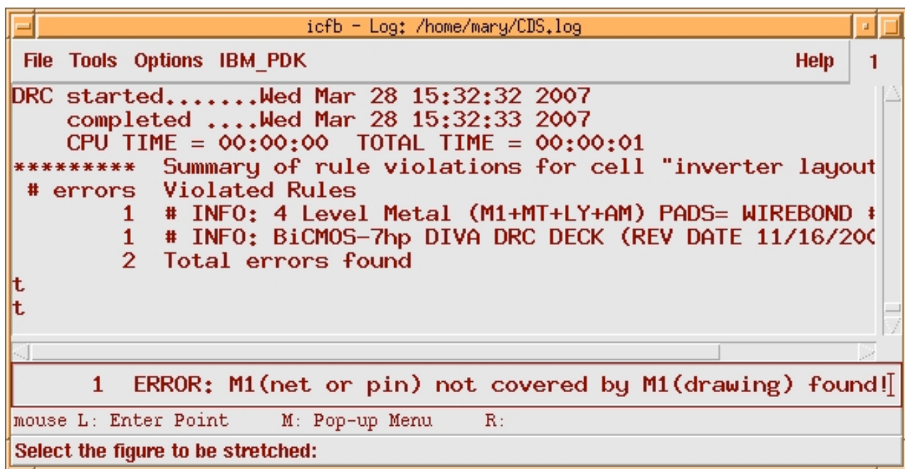
Figure 31- DRC check result in ICW
