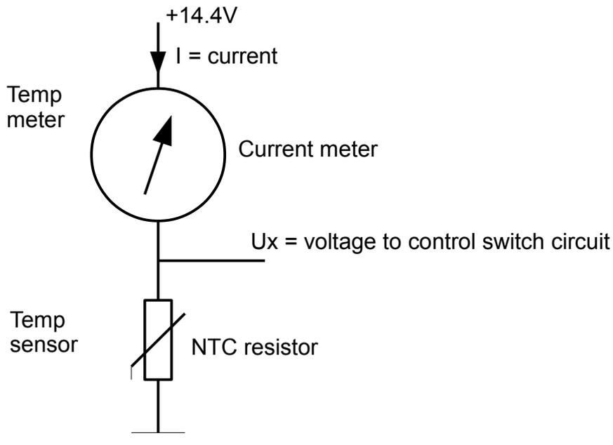
Working principle: Temperature rises  $\gg$  NTC resistance decreases  $\gg$  voltage  $U_x$  decreases  $\gg$  Current increases  $\gg$  Meter indicates higher temperature
