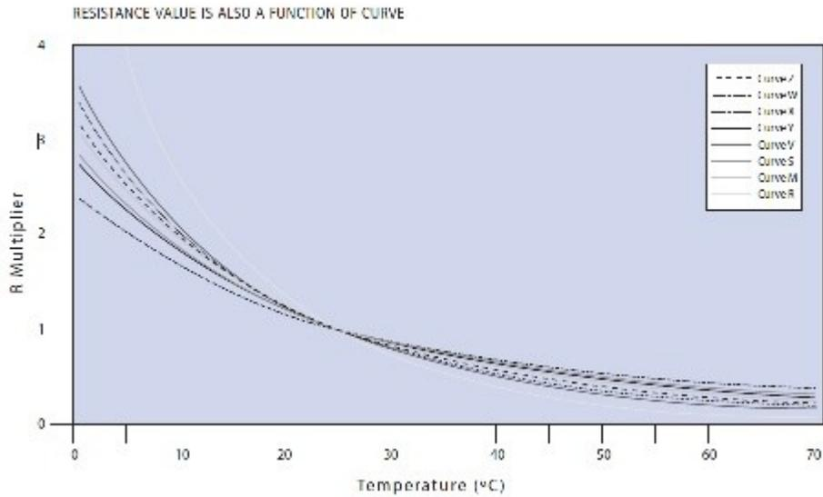
example of this is Quality Thermistors 'Z' curve it's by far the most common curve in the industry and most major thermistor manufacturers have a very similar curve offerings.
