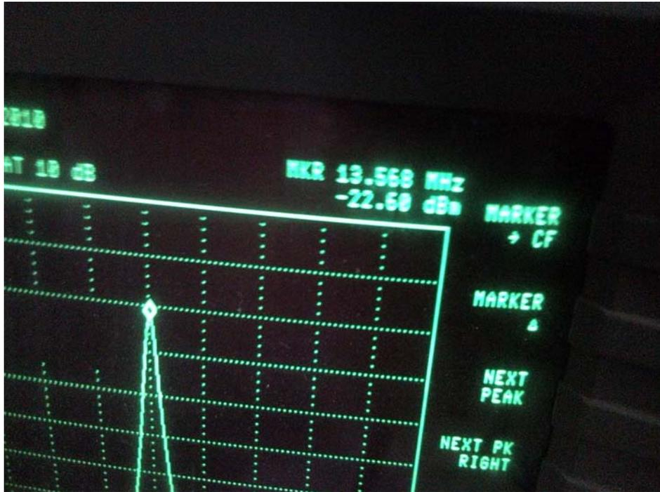
Now , I move the tag from area A to area B, and measure again, the inductive power is -22.46 dbm, but in this area the RFID reader can read or write the tag well.
