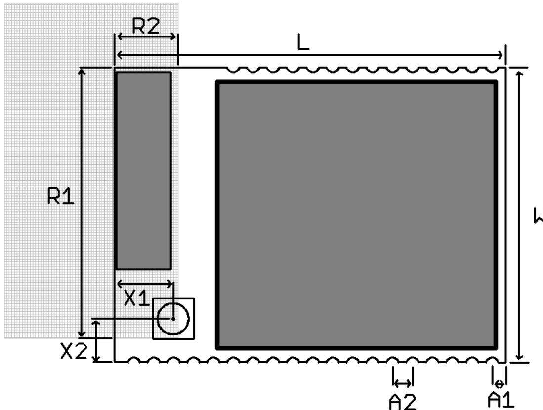
Figure 8. ETRX3 Physical Dimensions
