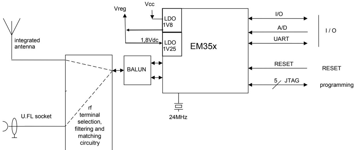
**Figure 2: Hardware Diagram**
