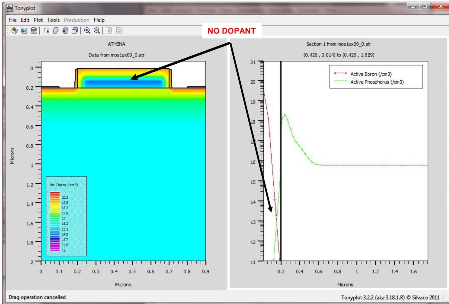
The only way to fix this is to dope the poly after it is deposited before etch.
