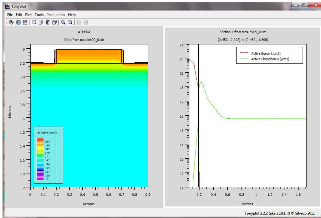
So this is more accurate, but there is a consequence of this increased accuracy. Without changing anything else, the VT has increased to almost 200mV. So the VT adjust implant will need to be fine tuned.
