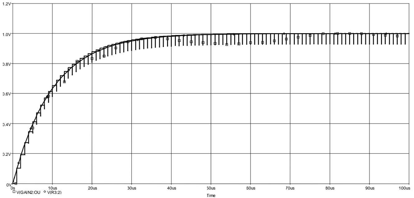
**Step response:** Active low pass 1<sup>st</sup> order (analog and S/C)
