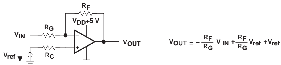
Figure 7. Inverting Amplifier
