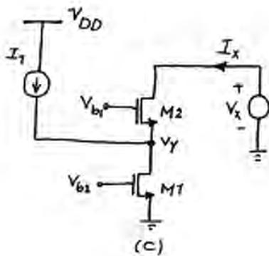
we assume  $V_{b1} > V_{b2}$  and both  $M_1$  and  $M_2$  operate in saturation region if  $V_x = V_{DD}$
