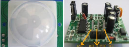
Motion detector module uses a motion detector IC and PCB mounted Fresnel lens.
