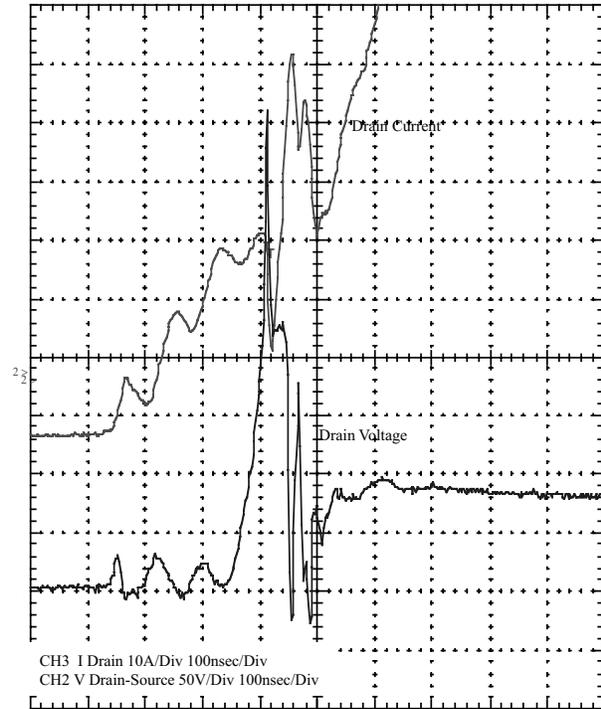
Fig. 8. MOSFET failure with short circuit load
