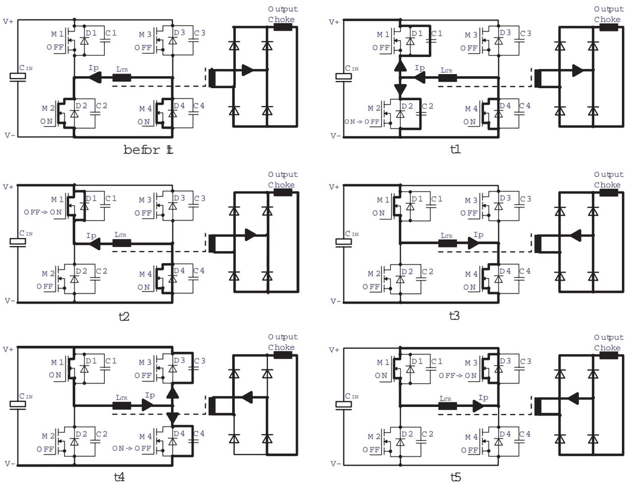
Fig. 5. Evolution of transformer current with time.
