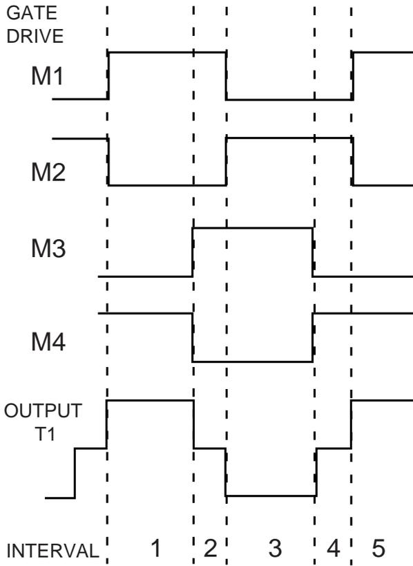
Fig. 4. Gate drive and T1 output voltage waveform.
