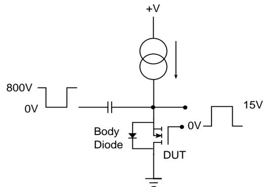
Fig. 16. Abbreviated schematic.
