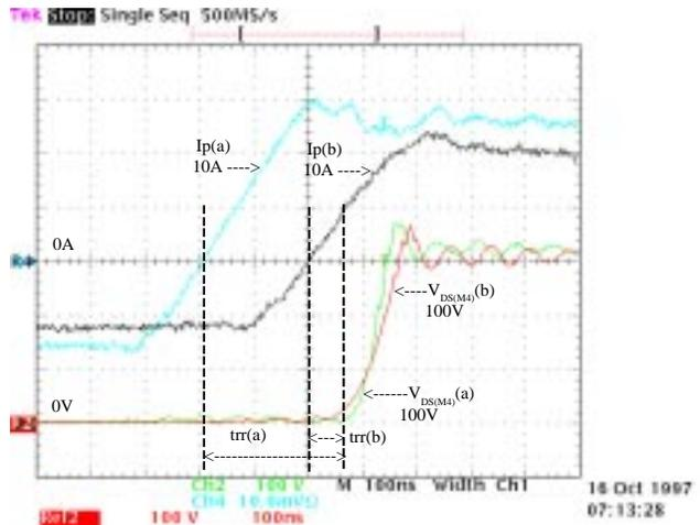
Fig. 9. Effect of additional capacitance with short-circuit load
