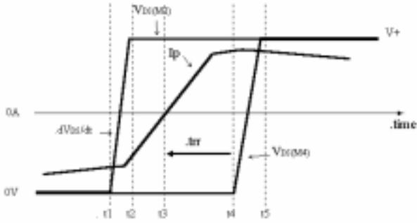
Fig. 6. Switch voltage and primary current relationship.
