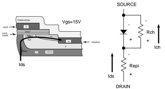
Fig. 14. Reverse current flow in the channel only.
