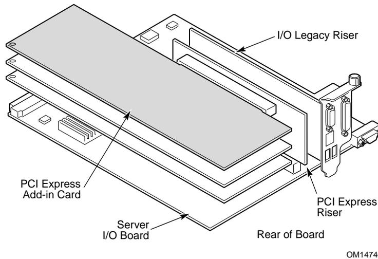
**Figure 1-2: Example Server I/O Board with PCI Express Slots on a Riser**
