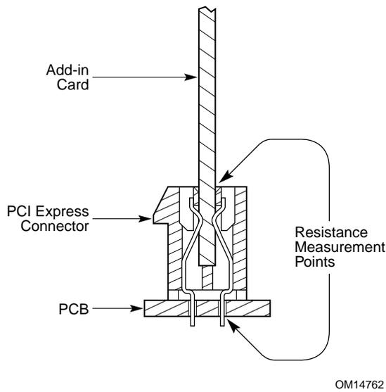
**Figure 5-5: Contact Resistance Measurement Points**
