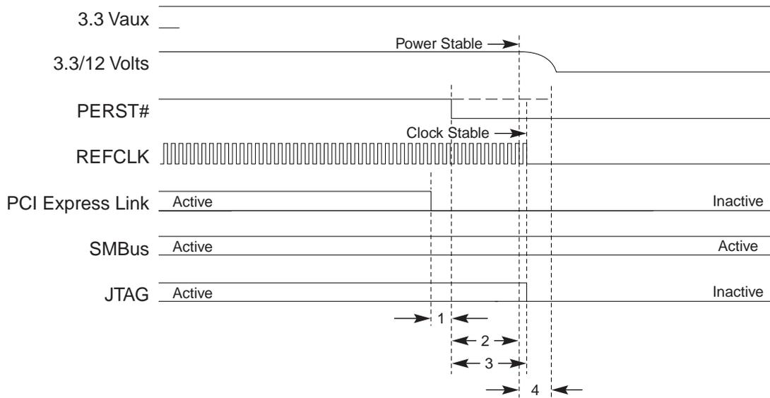
1. The PCI Express link will be put into an inactive state (Device in D3<sub>hot</sub>) prior to PERST# going active, except in the case of a surprise power down.
