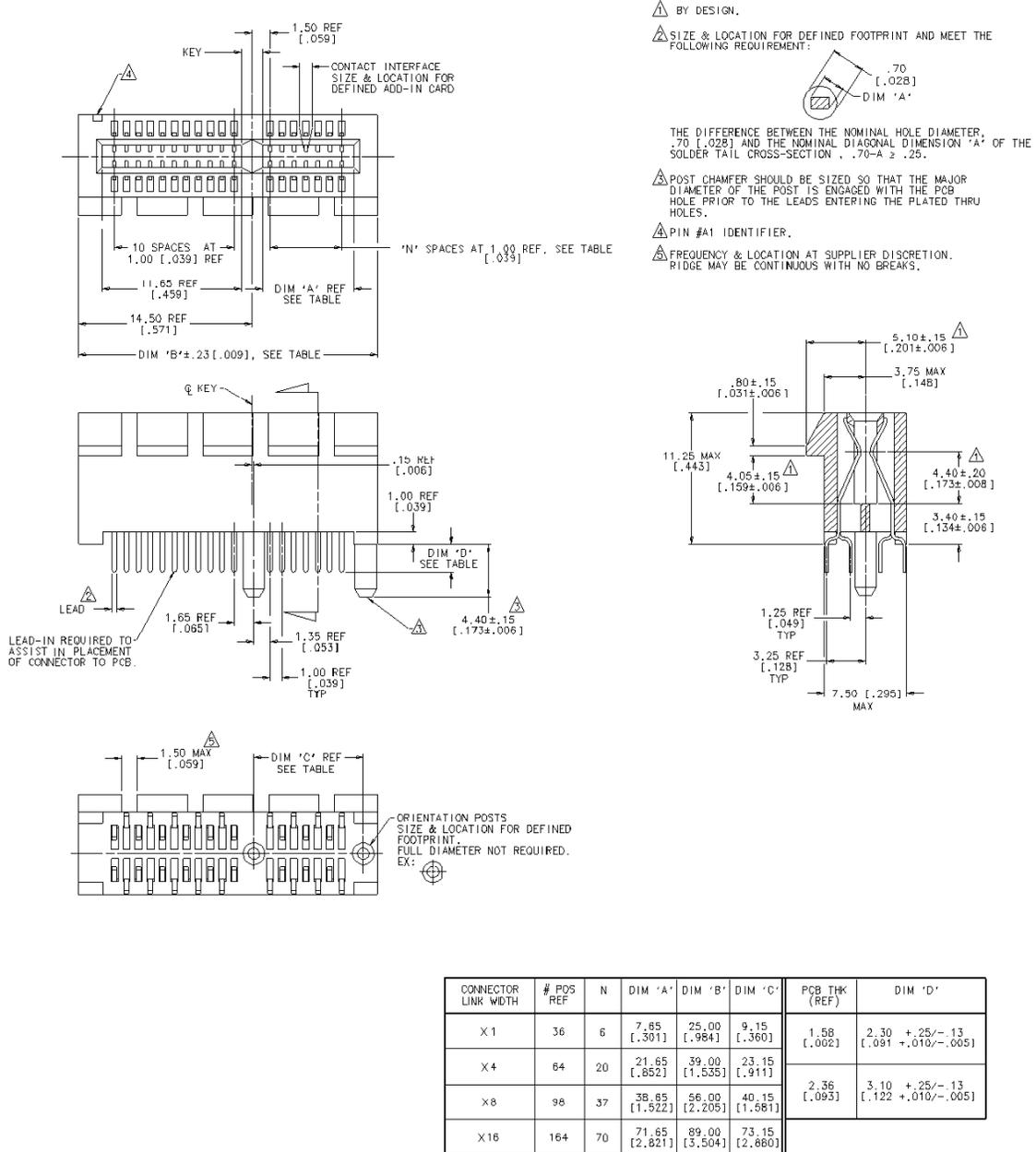
Figure 5-1: Connector Form Factor
