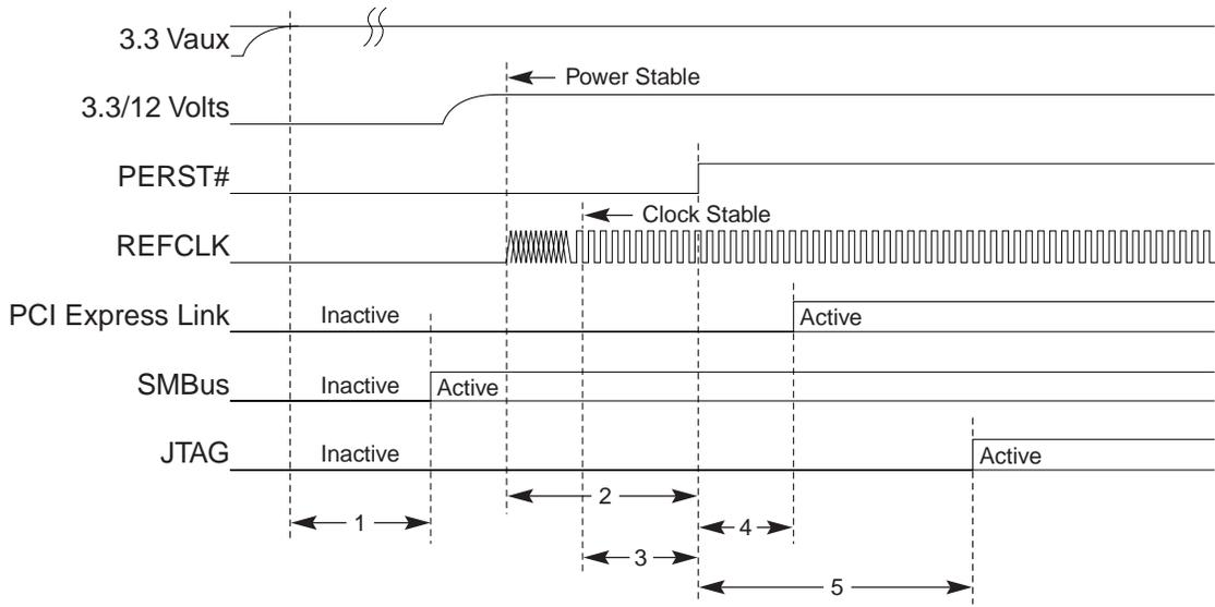
1. 3.3Vaux stable to SMBus driven (optional). If no 3.3Vaux on platform, the delay is from +3.3V stable
