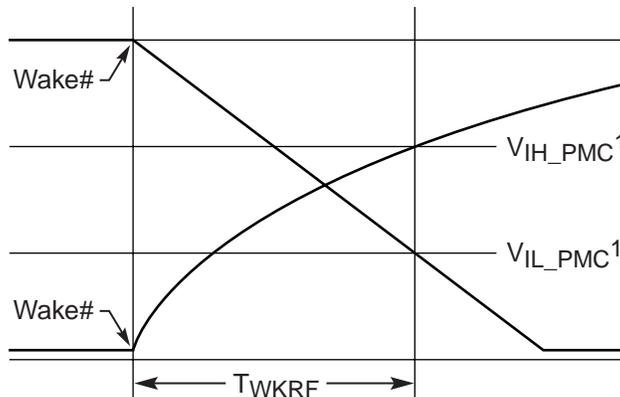
Note 1: Power Management Controller input switching levels are platform dependent and are not set by this specification.
