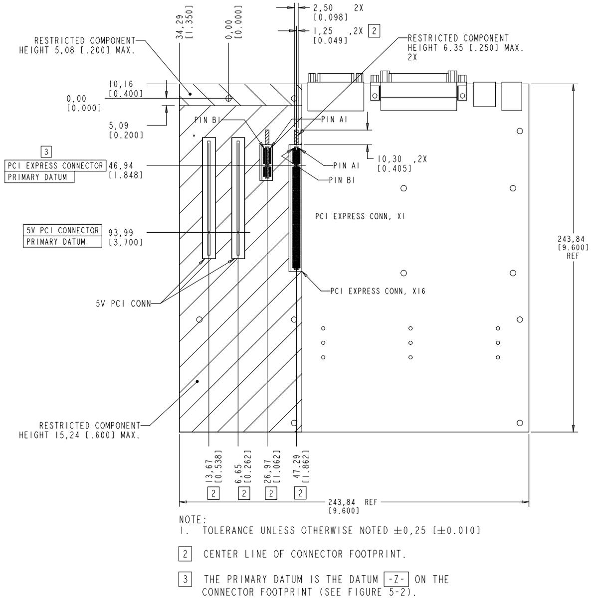
**Figure 6-14: PCI Express Connector Location in a microATX System with Two PCI Express Connectors**
