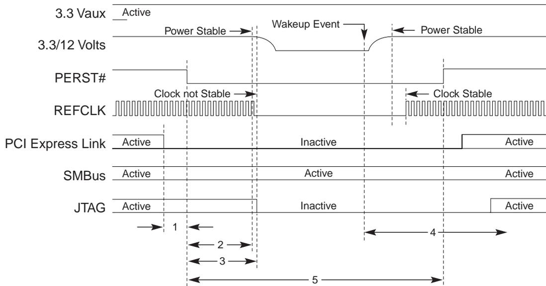
1. The PCI Express link will be put into electrical idle prior to PERST# going active.
