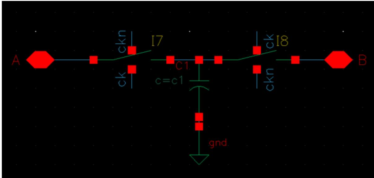
Because the capacitor transfers a fixed charge on each clock cycle, it is effectively a lossless resistor with a resistance of  $1/(Cf)$  where  $f$  is the switching frequency.
