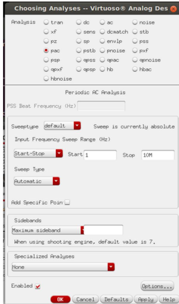
The PAC analysis is set up as for the AC analysis, as shown above. To set up the outputs, I used the calculator to create these expressions: Magnitude: `db20(v("/out" ?result "pac"))` Phase: `phase(v("/out" ?result "pac"))` -3dB point: `cross(db20(v("/out" ?result "pac")) -3 1 "either" nil nil)`
