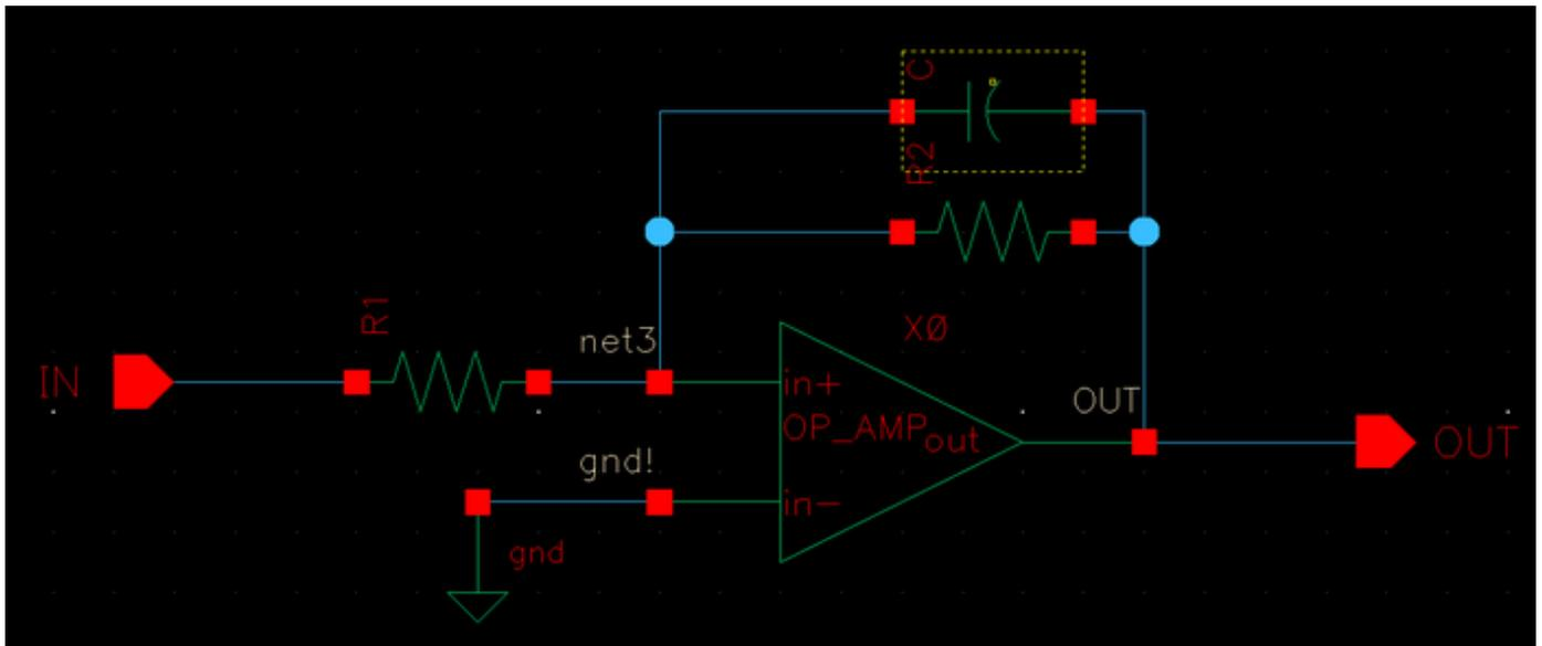
Above is shown a simple low pass filter. Its gain is  $R2/R1$ , so for 0dB gain,  $R2=R1$ . The -3dB frequency is  $1/(2\pi R2C)$ . Each resistor can be replaced with a switched capacitor like below.
