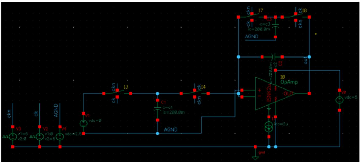
Setting  $c1=c3=1\text{pF}$ ,  $f=100\text{kHz}$  (nb switching frequency needs to be considerably larger than the cut off frequency, say 10X or more) and  $c2=16\text{pF}$  should give the required filter.
