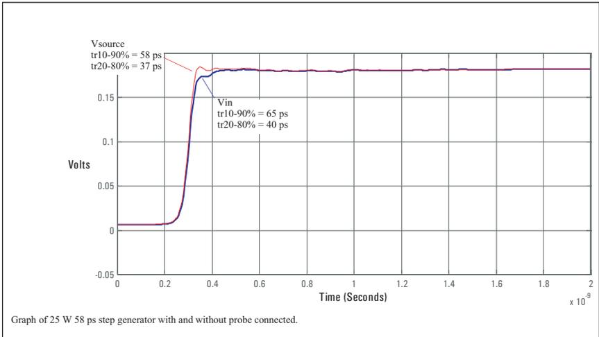
Figure 5. Time-domain loading for N5381A solder-in probe head
