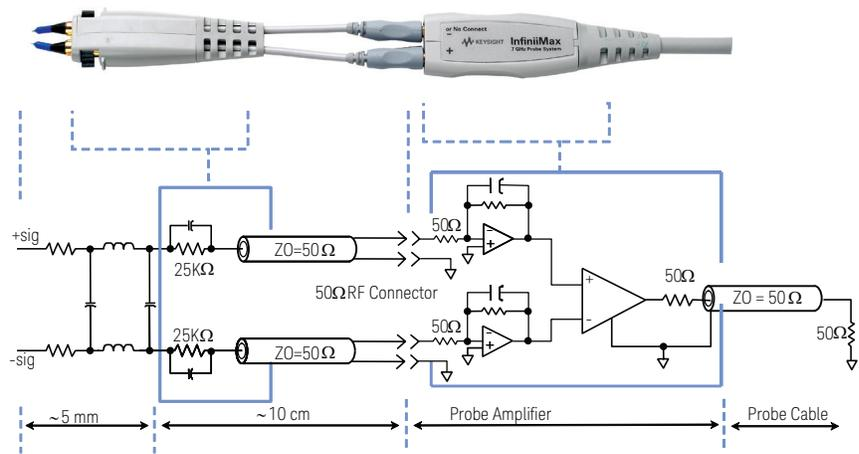
Figure 1. InfiniiMax architecture
