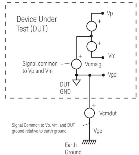
Figure 10 A differential signaling system to be measured
