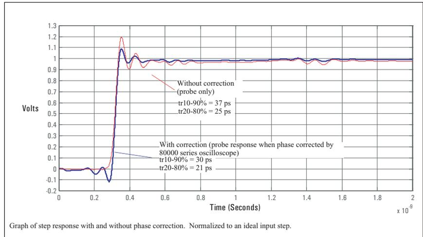
Figure 3. Time domain response of N5381A solder-in probe head and 1169A probe amplifier
