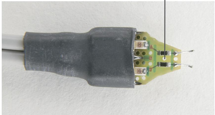
Figure 2. InfiniiMax solder-in probe head detail
