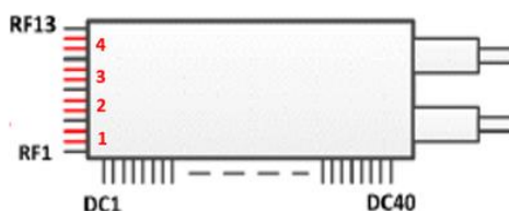
Figure 6 RF and DC signal orientation
