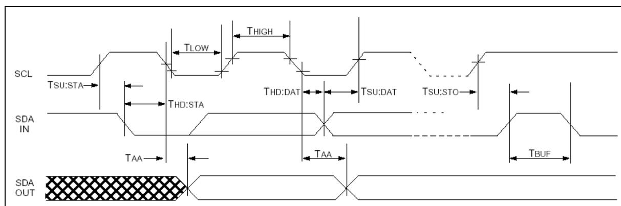
Figure 1.1 - I<sup>2</sup>C bus timing
