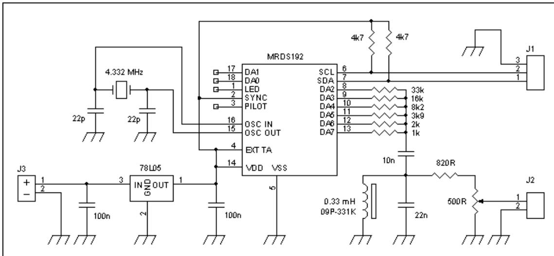
Figure 6.1 - Sample application circuit - schematic diagram
