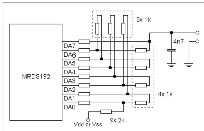
Figure 3.4 - 8-bit D/A converter R/2R network
