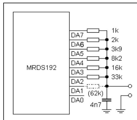
Figure 3.3 - 6 (or 7) bit D/A converter network
