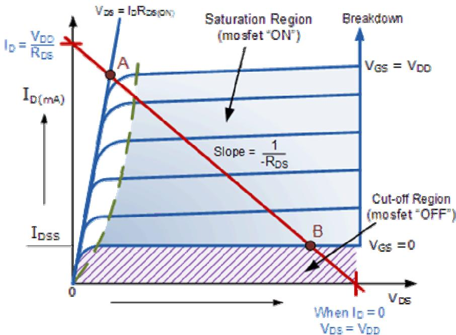
The minimum ON-state gate voltage required to ensure that the MOSFET remains fully-ON when carrying the selected drain current can be determined from the V-I transfer curves above. When  $V_{IN}$  is HIGH or equal to  $V_{DD}$ , the MOSFET Q-point moves to point A along the load line.
