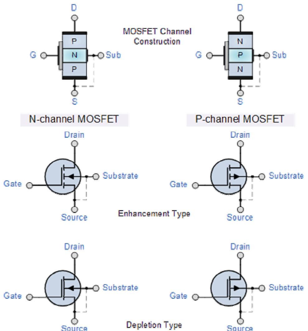
channel line is shown dotted or broken it is an "Enhancement" (normally open) type MOSFET. The direction of the arrow indicates either a P-channel or an N-channel device.
