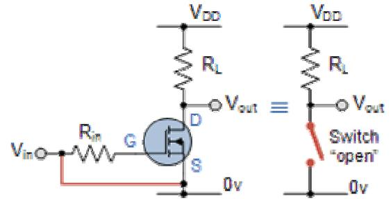
Then we can define the "cut-off region" or "OFF mode" of a MOSFET switch as being, gate voltage,  $V_{GS} < V_{TH}$  and  $I_D = 0$ . For a P-channel MOSFET, the gate potential must be negative.
