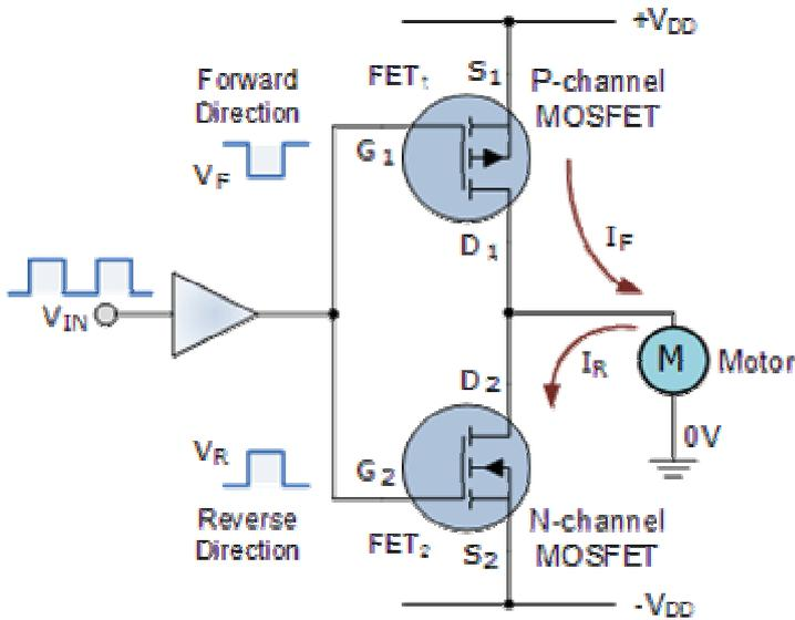
The two MOSFETs are configured to produce a bi-directional switch from a dual supply with the motor connected between the common drain connection and ground reference. When the input is LOW the P-channel MOSFET is switched-ON as its gate-source junction is negatively biased so the motor rotates in one direction. Only the positive +VDD supply rail is used to drive the motor.
