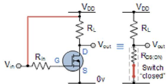
Then we can define the "saturation region" or "ON mode" of a MOSFET switch as gate-source voltage,  $V_{GS} > V_{TH}$  and  $I_D = \text{Maximum}$ . For a P-channel MOSFET, the gate potential must be positive.
