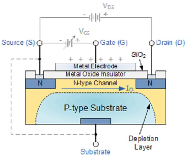
The construction of the Metal Oxide Semiconductor FET is very different to that of the Junction FET. Both the Depletion and Enhancement type MOSFETs use an electrical field produced by a gate voltage to alter the flow of charge carriers, electrons for N-channel or holes for P-channel, through the semiconductive drain-source channel. The gate electrode is placed on top of a very thin insulating layer and there are a pair of small N-type regions just under the drain and source electrodes.
