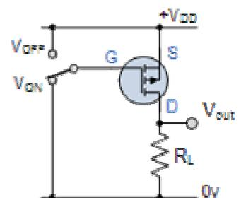
In a P-channel device the conventional flow of drain current is in the negative direction so a negative gate-source voltage is applied to switch the transistor "ON". This is achieved because the P-channel MOSFET is "upside down" with its source terminal tied to the positive supply +VDD. Then when the switch goes LOW, the MOSFET turns "ON" and when the switch goes HIGH the MOSFET turns "OFF".
