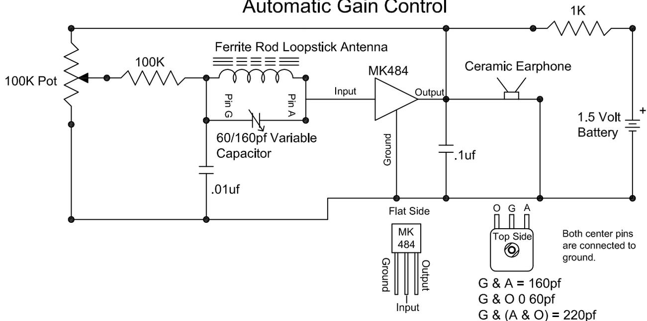
The automatic Gain control provided by the 100K resistor and 100K pot. Using this added pot there is no need to vary the value of the 1K resistor to prevent oscillations. The 100K pot is not sold with the kit. It can be purchased separately.
