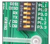
**Figure 8-4:** Switch 8 on the DIP switch SW8 is in the ON position, DS1820 is connected to the P3.3 pin
