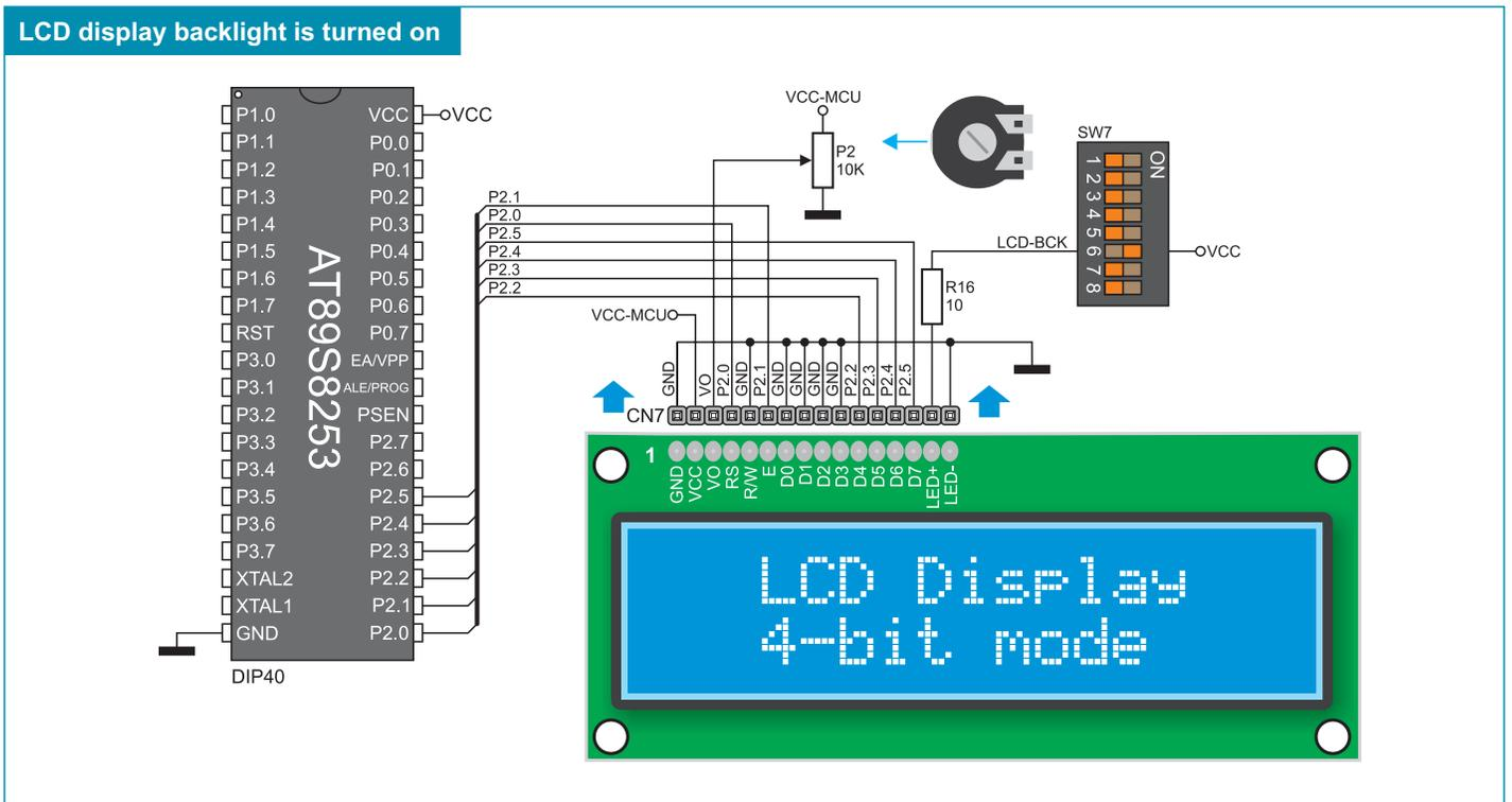
Figure 14-3: Alphanumeric 2x16 LCD display connection schematic
