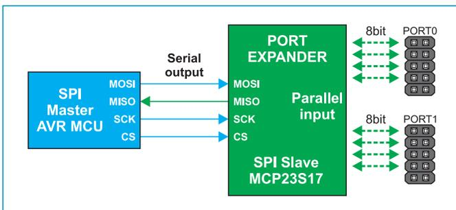
Figure 18-3: SPI communication block diagram
