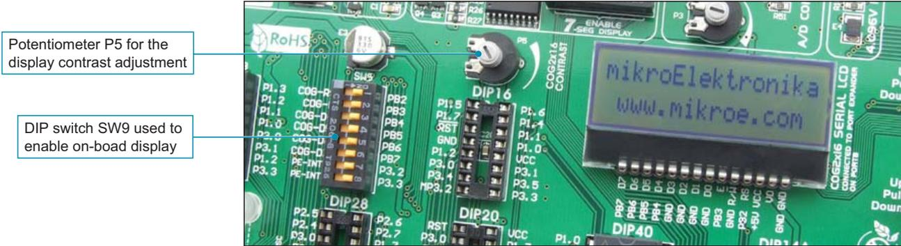
Figure 13-1: On-board 2x16 LCD display
