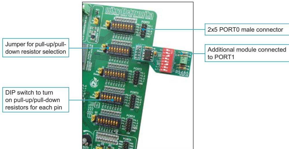
Figure 17-1: I/O ports
