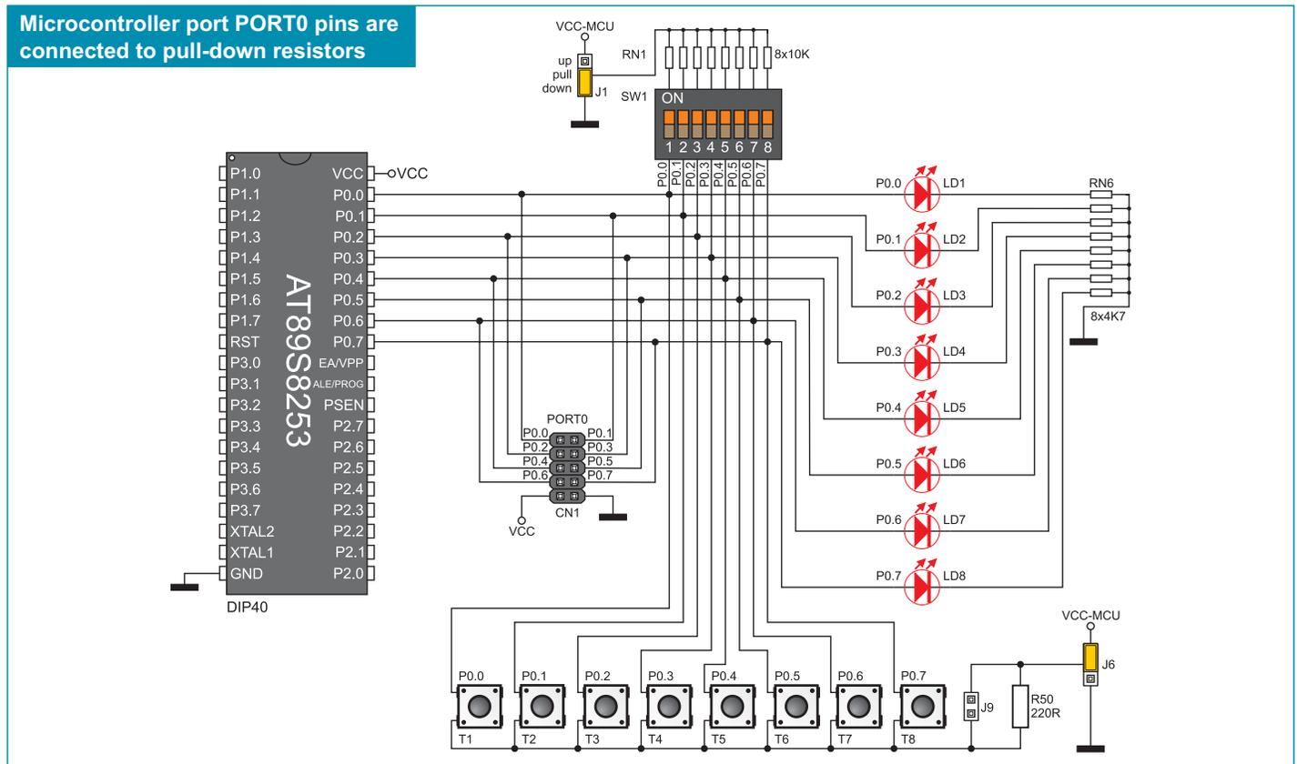
Figure 17-4: Port PORT0 connection schematic
