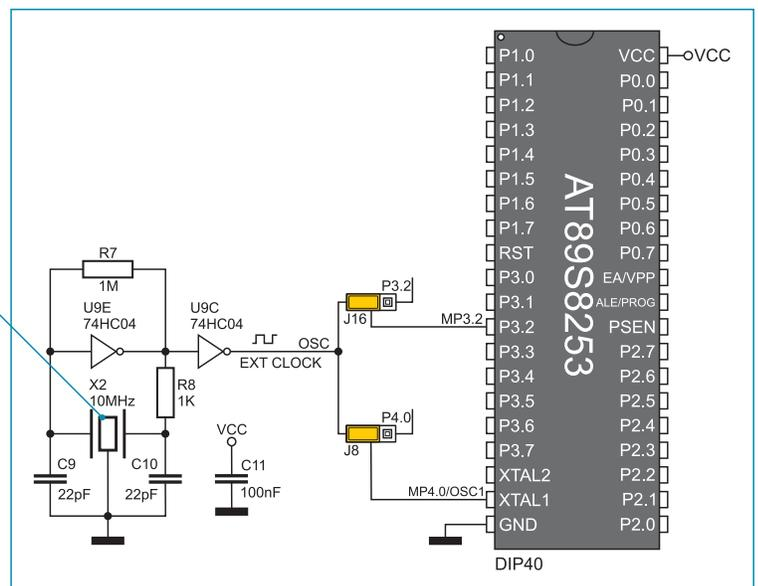
Figure 4-2: Oscillator schematic
