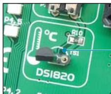
**Figure 8-2:** DS1820 is plugged into the connector
