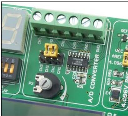
Figure 7-1: ADC (jumper default position)
