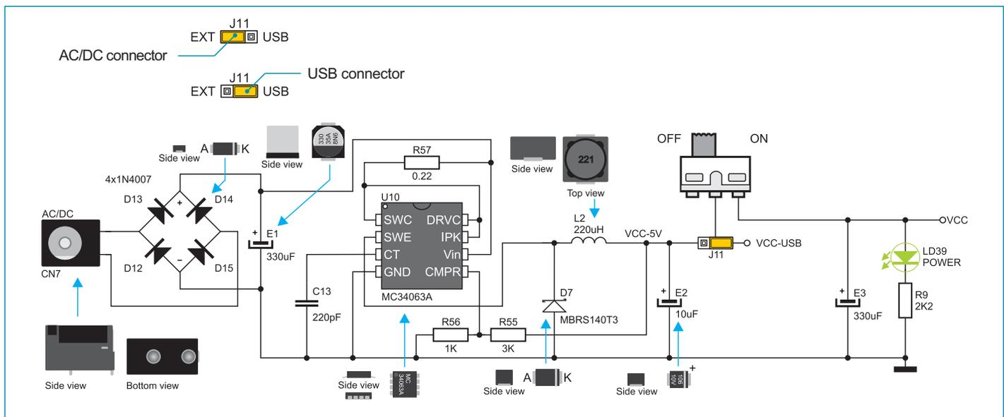
Figure 5-2: Power supply source connection schematic
