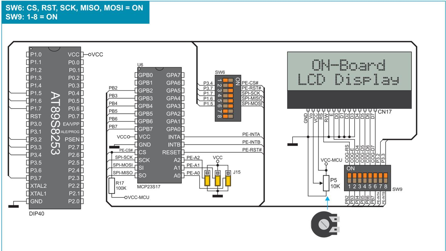
Figure 13-2: On-board LCD display connection schematic
