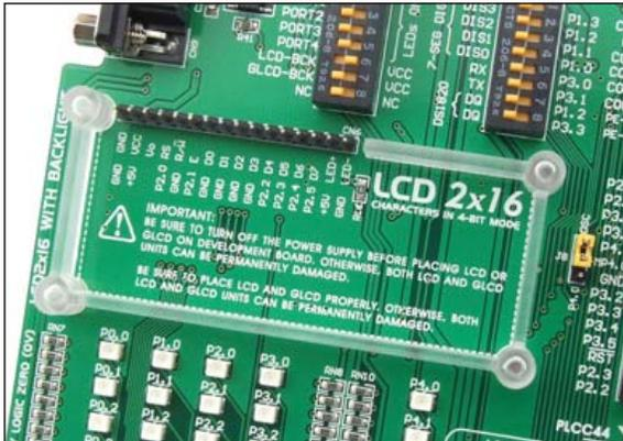
Figure 14-1: Alphanumeric 2x16 LCD display connector
