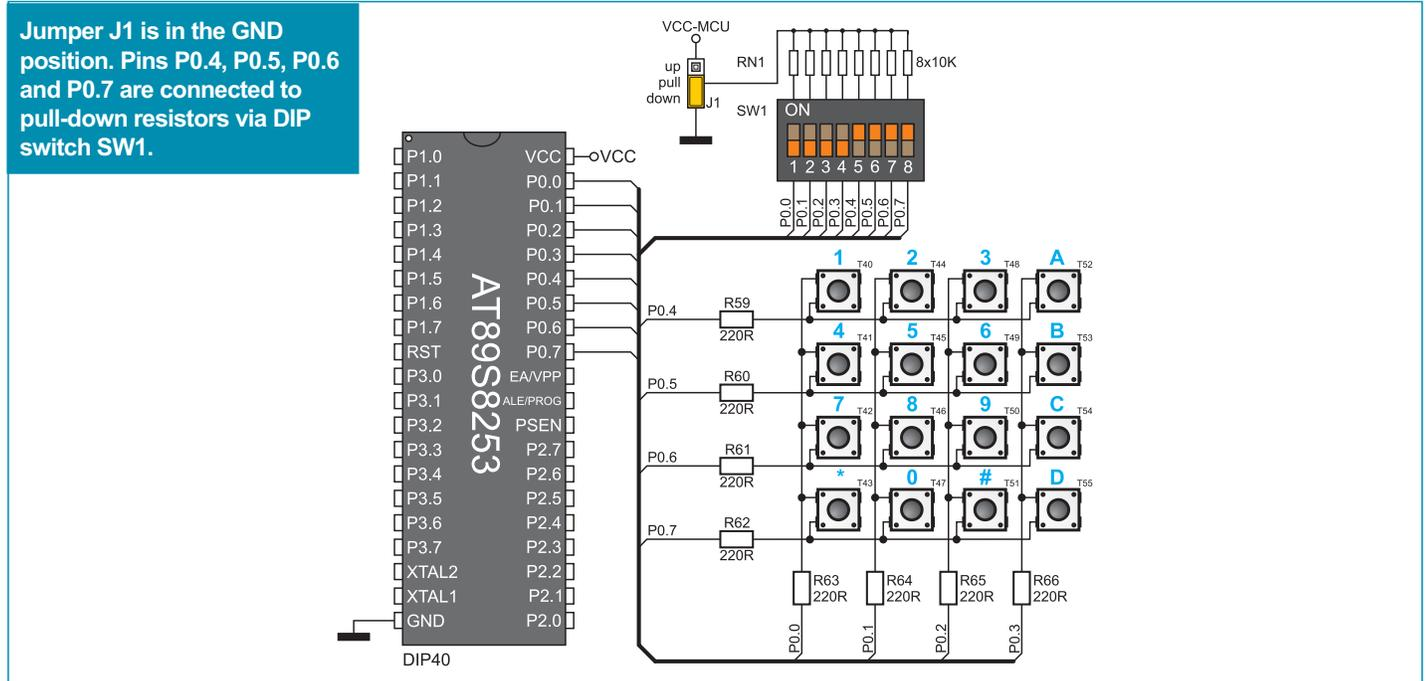
Figure 12-3: 4x4 keypad and microcontroller connection schematic
