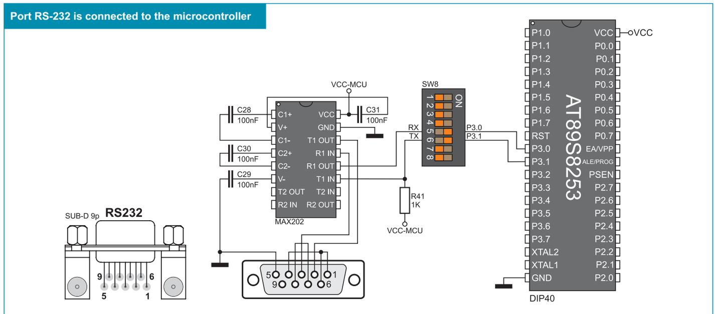
Figure 6-2: RS-232 module schematic
