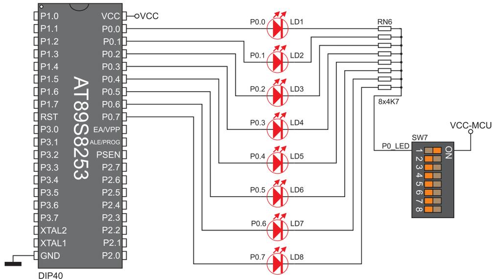
Figure 9-2: LED diode and port PORT0 connection schematic
