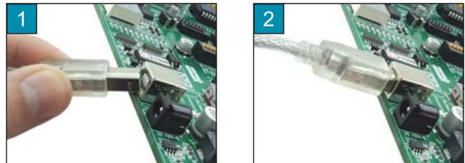
Figure 1-2: Connecting USB cable
