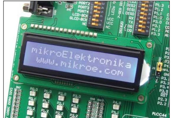
Figure 14-2: Alphanumeric 2x16 LCD display
