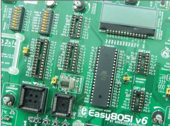
Figure 2-1: Microcontroller sockets
