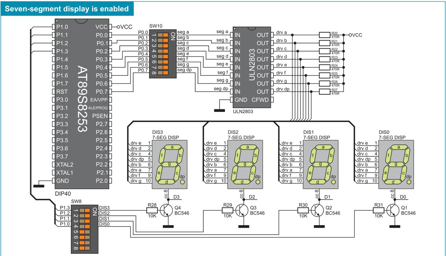
Figure 16-4: Seven-segment display connection schematic
