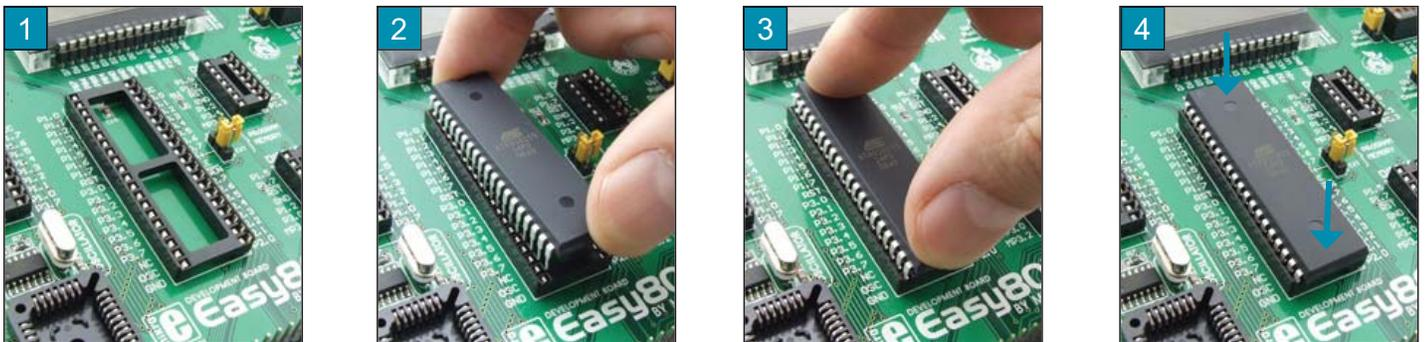
Figure 2-2: Plugging a microcontroller into appropriate socket
