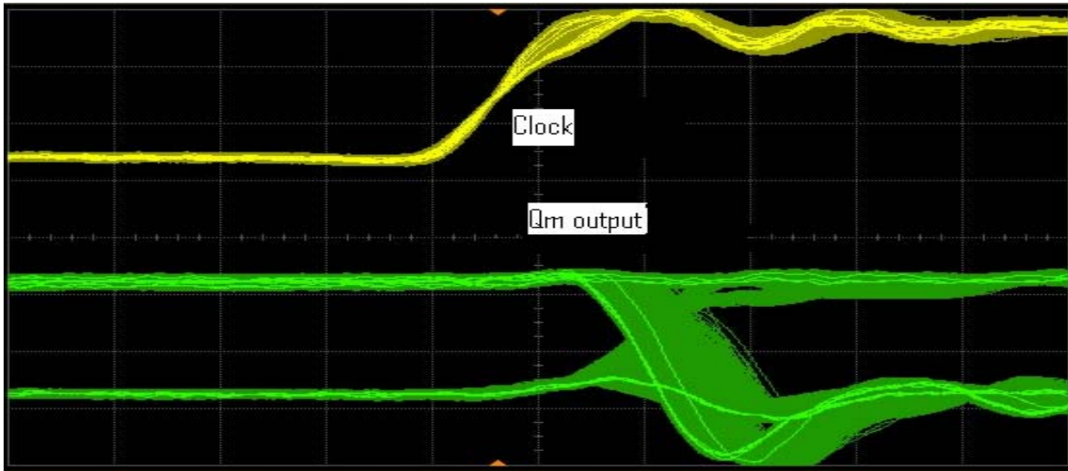
Fig 9 Master flip-flop output when control voltage V3 is 1V and frequency is 15MHz
