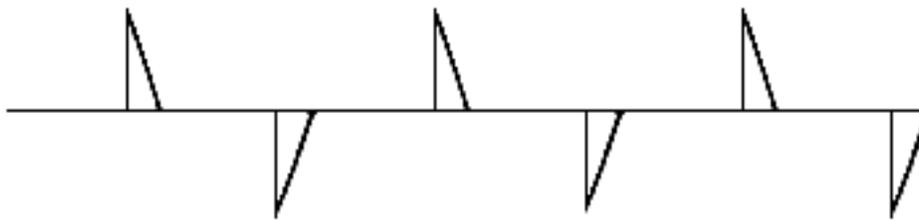
This is usually used for light dimming because lights are resistive loads, and will not flicker even if they only get voltage spikes as in the last waveform. This method does not work well for inductive loads because they usually require a 'nicer' sine wave than what is shown here, and there may be some inductive kickback current which will not allow the TRIAC to turn off.
