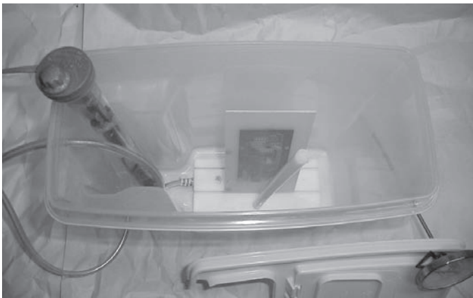
Figure 5-8: Inside view of etchant tank
