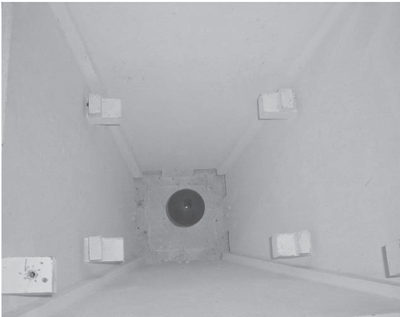
Figure 6-5: Exposure cone cleat placement
