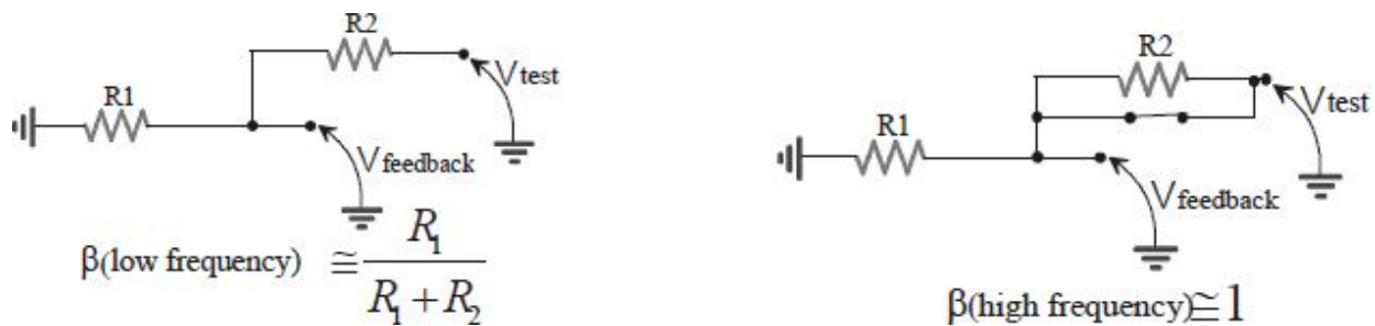
Fig. 3.65: Feedback block at low (on the left) and high frequencies (on the right).
