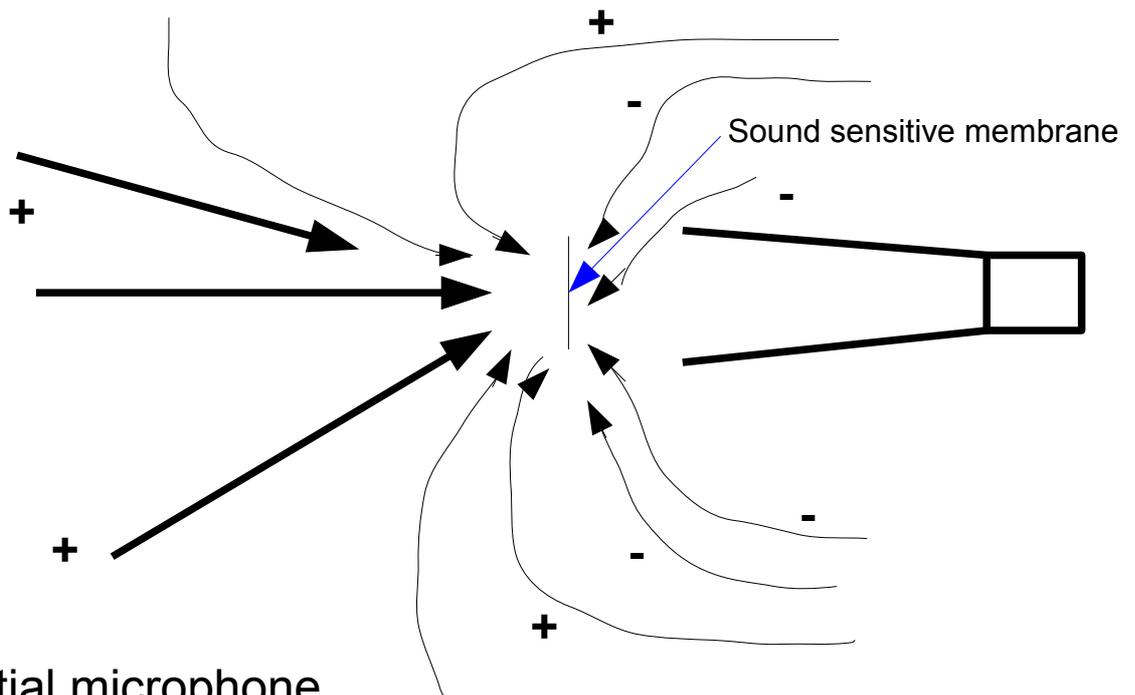
Differential microphone construction attenuates sounds from rear and side
