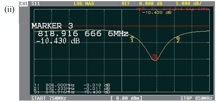
Fig. 7. Input return loss of microstrip dipole antenna from 750 MHz – 850 MHz.
