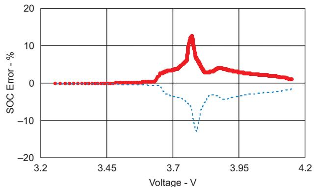
Fig. 5b. Error in SOC estimation depending on voltage where estimation was performed.
