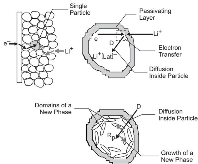
Fig. 1a. Simple steps of Li-ion battery-discharge kinetics.
