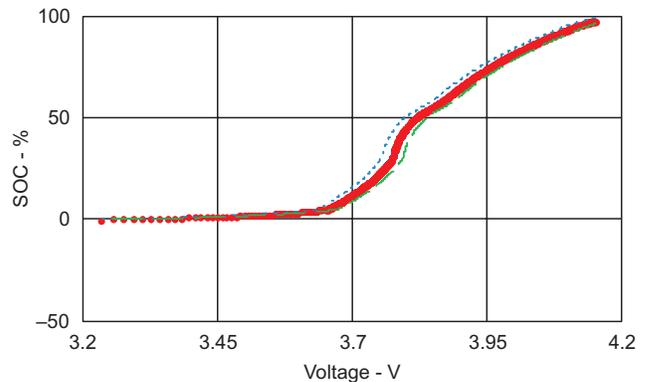
Fig. 5a. SOC vs. voltage with indicated confidence interval resulting from transient error.
