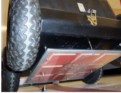
Figure 3.3.1: Protected Capaciflector Grid Attached to Rover
