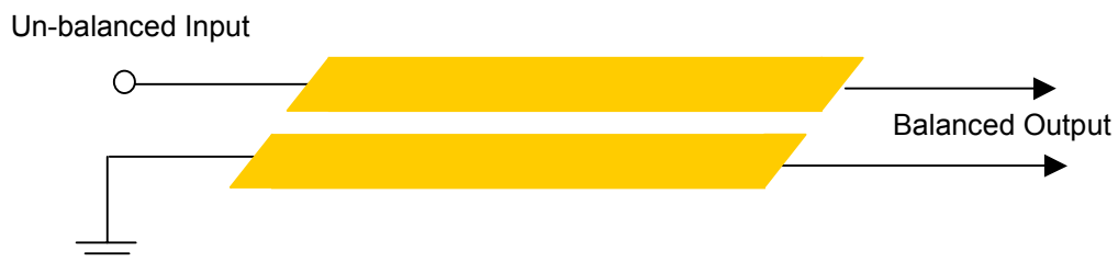
Figure 6 Simple coupled line balun
