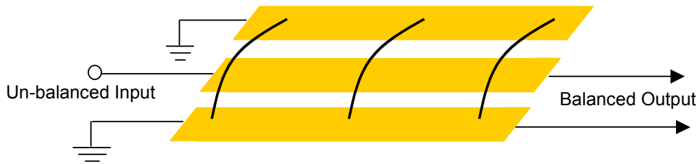
Figure 7 Coupled line balun using multiple coupled lines
