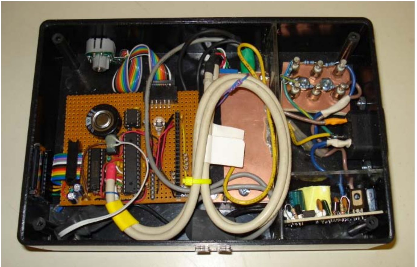
The digital board, power supply, input voltage divider, etc.
