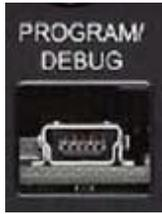
7. For enhanced demonstration, the application requires the Real-Time Data Monitor (RTDM). Users can connect a mini-USB cable from their computer to the J6 connector of the dsPICDEM MCHV-2 Development Board.
