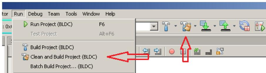
5. After a successful build, download the code to the dsPICDEM MCHV-2 Development Board by selecting the “Make and Program the device main project” button on the toolbar.
