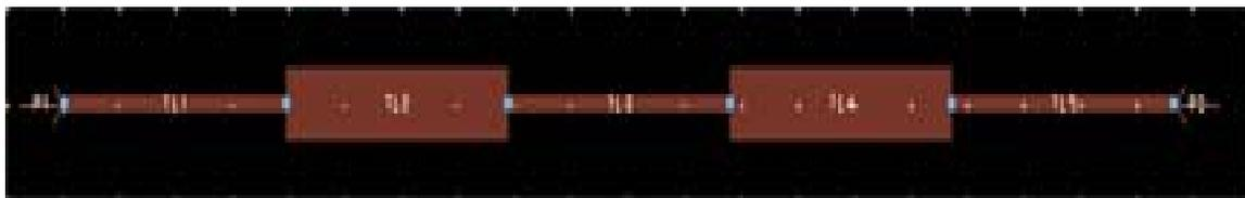
However, this step has just generated the top view of the filter, i.e. the information of “L” and “W”, so we also need to specify the substrate information separately. A convenient way is to transfer the substrate information from the schematic sheet to this layout sheet, this can be done by click the “momentum” button on the top menu in the layout window and select “Substrate” > “Update from schematic”. Before we do the simulation, we need to set up the mesh, which is an
