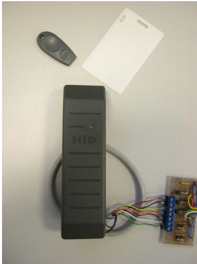
Figure 7. MiniProx™ proximity card reader and two transponders: the key fob and the ISO card
