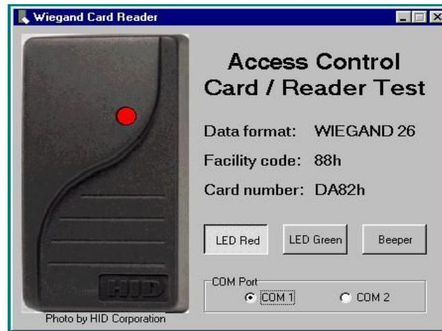
Figure 12. Read-out of Wiegand 26 card data
