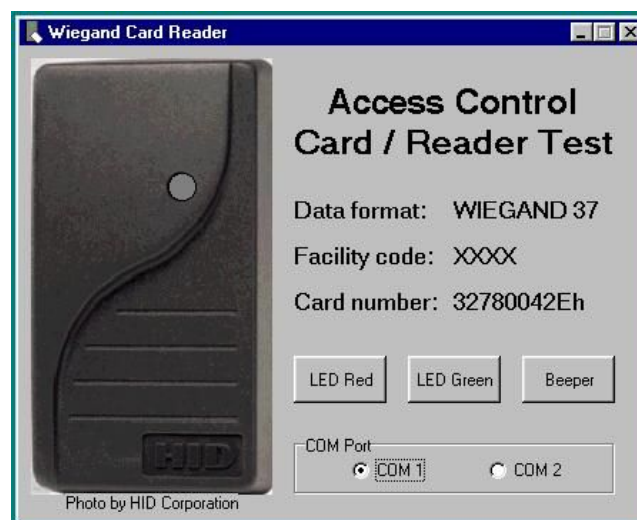
Figure 13. Read-out of Wiegand 37 card data
