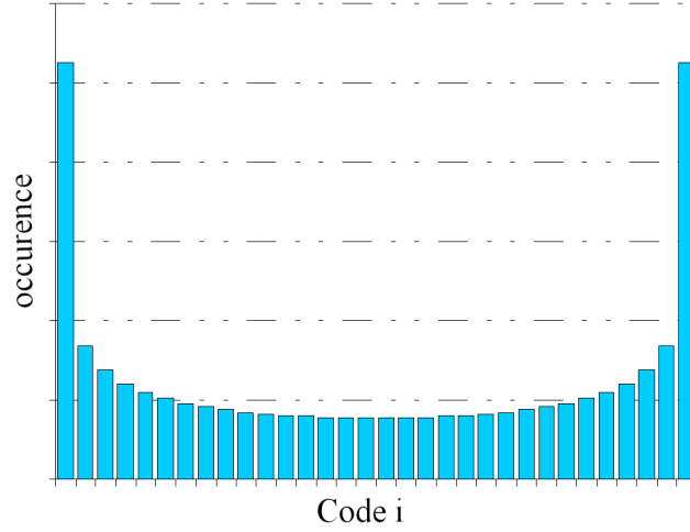
Figure 6.1 : Histogram with an overrange sinus signal.
