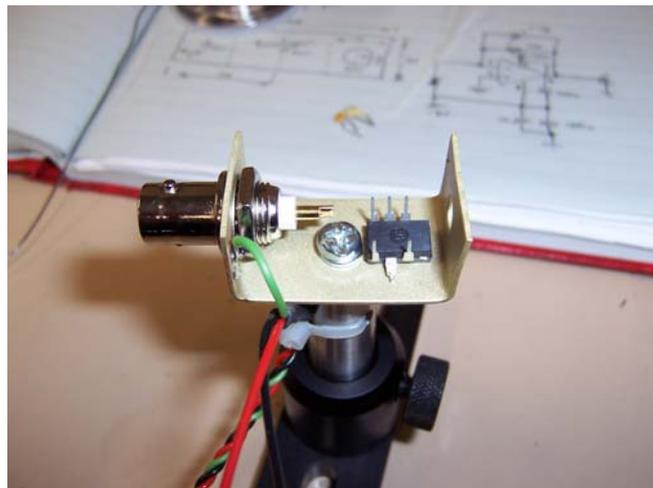
This photo illustrates the op-amp ready to be soldered, with pin 3 soldered straight down to the chassis. Because of the relatively thick metal I used, this requires a *lot* of heat – be careful not to incinerate the op-amp or your fingers. Note that I clipped off the unused pins of the op-amp to make things a little less cluttered. The wires cable-tied to the post run off to the connector for our power supplies.
