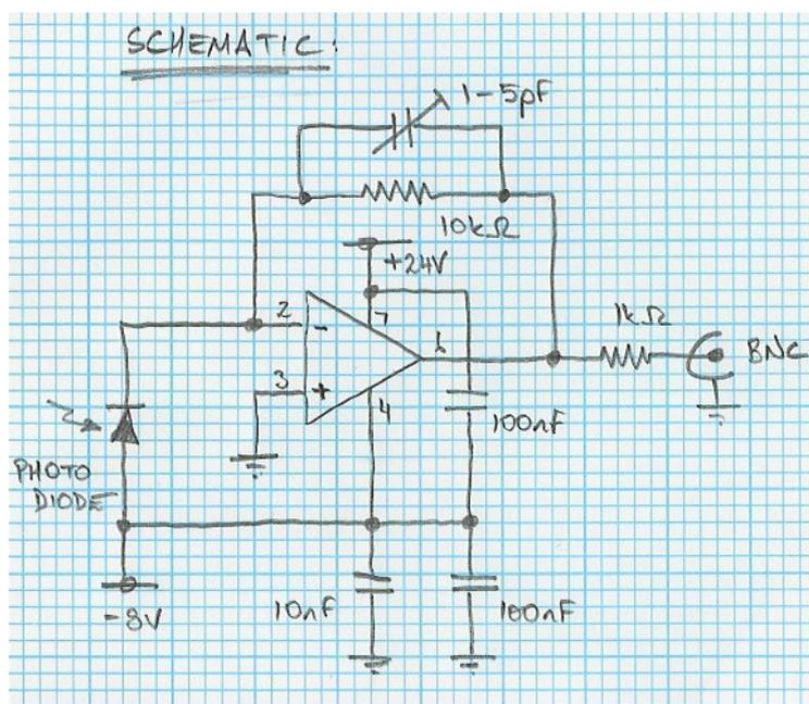
The only two components that rate a special mention are the 1-5pF variable feedback capacitor and the 1kΩ output resistor. The feedback capacitor compensates for the
