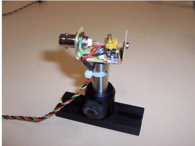
Voila! The completed unit! The photodiode can be seen protruding from the hole on the right and the yellow compensation capacitor was placed last to allow easy adjustment – now the moment of truth...
