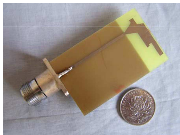
Fig. 6. Prototype of the proposed multiband antenna. (Color version available online at: http://ieeexplore.ieee.org .)
